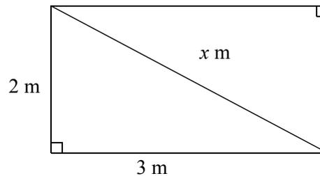
The brace should be 3.606 m to the nearest millimetre (3 606 mm).
