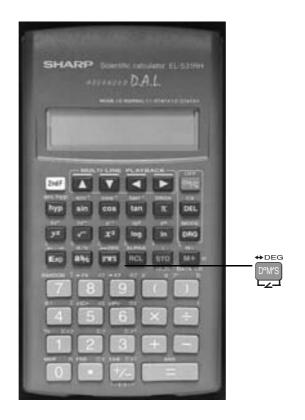
This key can be used for problems involving degrees, minutes and seconds or hours, minutes and seconds.
